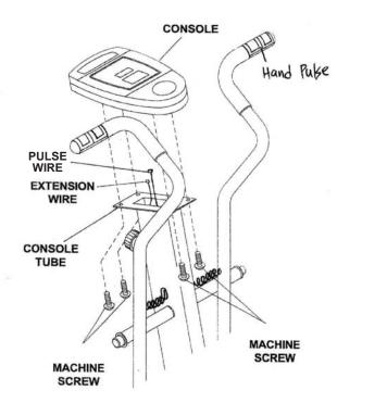
**12.** Remove the four MACHINE SCREWS from back of CONSOLE. Carefully plug EXTENSION WIRE and PULSE WIRE into bottom of CONSOLE. Attach CONSOLE to CONSOLE TUBE with MACHINE SCREWS from CONSOLE.
